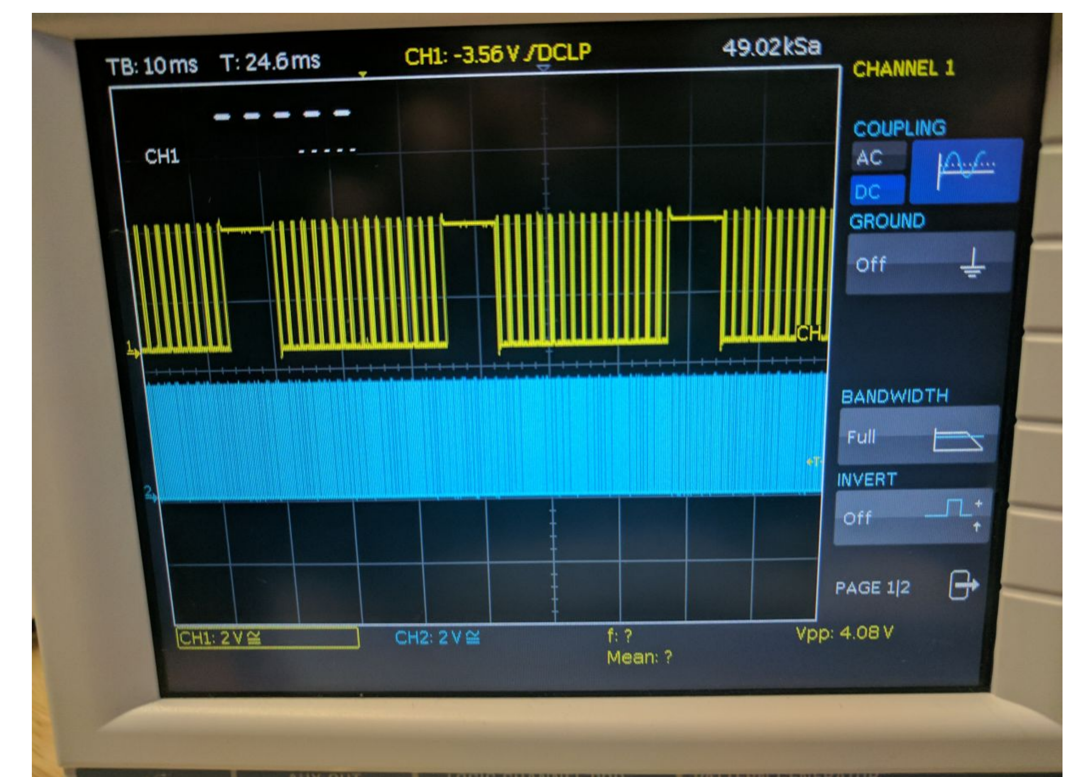
Pictured: analog to digital audio sampling in blue and sd-card write cycles in yellow
