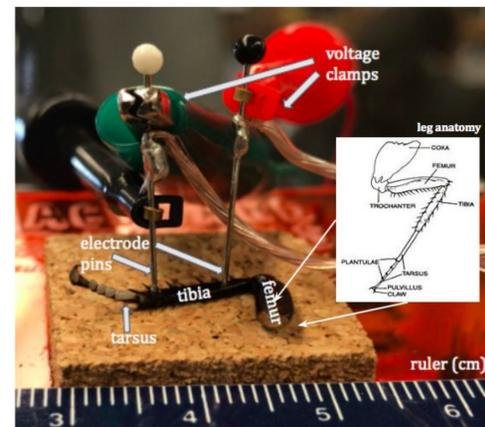
Figure 1 . Experimental Setup and Leg Anatomy of the Cockroach
